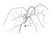
Insert the plain end of the cable through one side of the adjustable fastener. Loop the wire through the hole in the mounting profile and around the edge of the mounting profile at the predetermined locations. Re-insert the plain end of the cable through the remaining side of the adjustable fastener.
