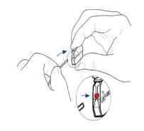
Feed swaged wire through tip of 'wire adjuster' (as shown). Push button (shown in grey) to adjust wire length. Release the button to lock in place.
