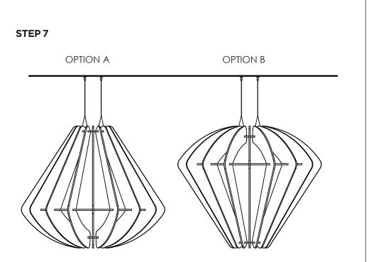
Re-adjust wire length as explained in STEP 5 until cloud hangs level. Note, there are 2 orientation options as shown below. STEP 8
