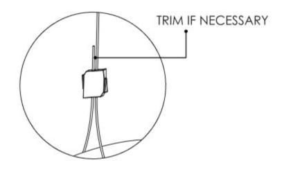
Once the Cloud is properly suspended, trim the excess cable. The cable is adjustable by depressing tab on appropriate side.
