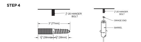
Install the 1/4"-20 hanger bolts to the substrate. The supplied hanger bolts are intended for use in wood only. For other substrates the installer will need to source the appropriate hardware.
