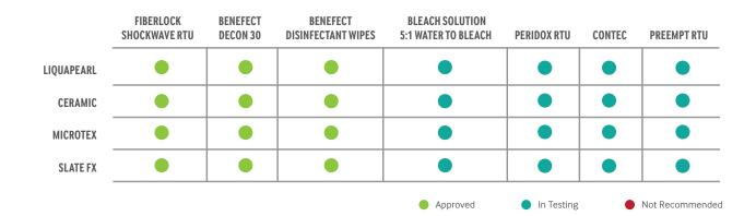
MDC Wall recommends these coatings for use with these EPA List N disinfectants for the best performance in areas requiring frequent disinfecting. We have tested these disinfectants but many others are available. Our testing has not revealed a hard surface disinfectant that harms MDC Wall coatings.
